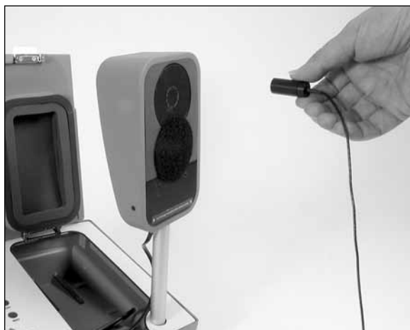
Figure 3.8.2B—Hold microphone six inches from the speaker
